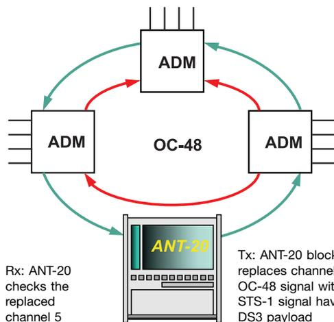
Ring test with Block & Replace
