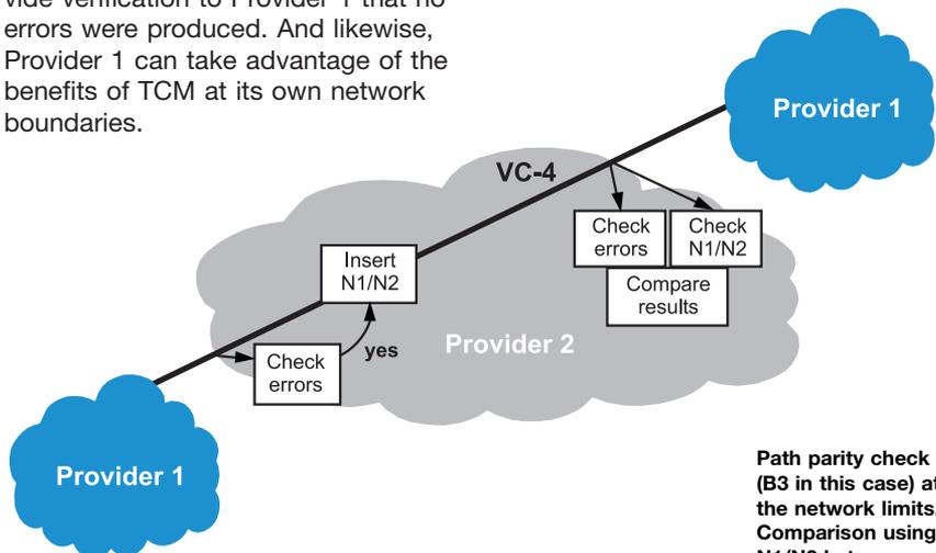
Path parity check (B3 in this case) at the network limits. Comparison using the N1/N2 bytes.
