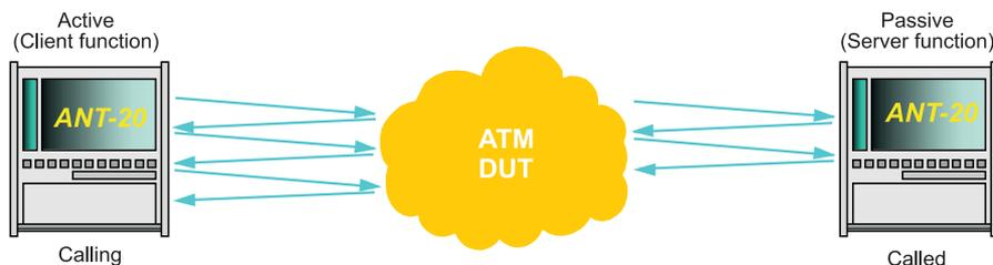
In *Called* mode, the ANT-20 with the BAG module can accept up to four calls simultaneously. Test scenarios involving five ANT-20/BAGs are thus possible.
