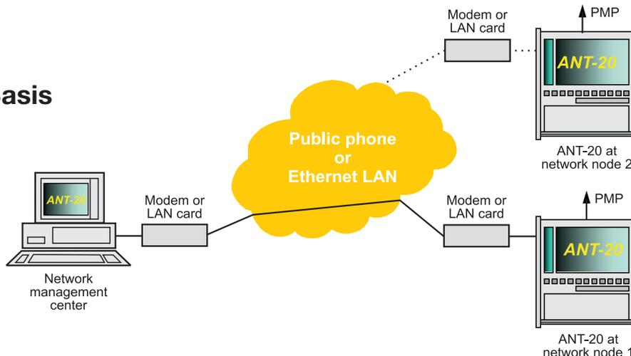
connected to a protected monitor point (PMP). By using test point scanners at the nodes, it is possible to connect a single ANT-20 to multiple PMPs. Via remote operation, a user at a network management center can now connect to each ANT-20.
