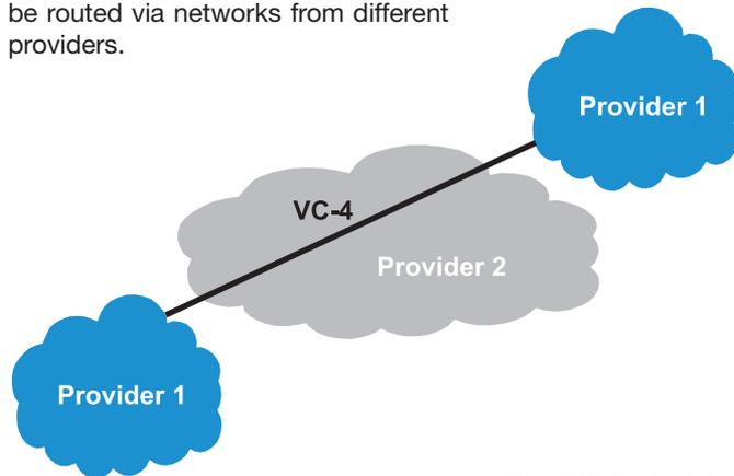
Provider 1 leases transmission capacity (a transparent STM-1/VC-4 "leased line") from Provider 2 to connect two subnetworks.
