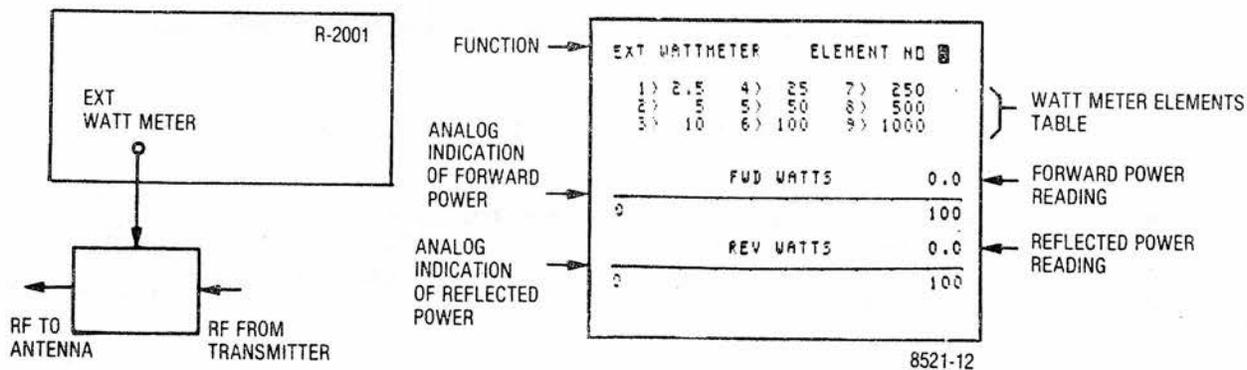
Figure 4-7. Wattmeter Test Setup and CRT Display
