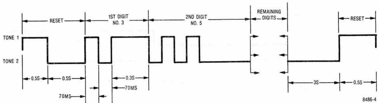
Figure 1-5. MTS Sequence Timing
