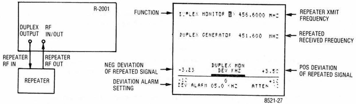
Figure 4-5. Duplex Generation Test Setup and CRT Display
