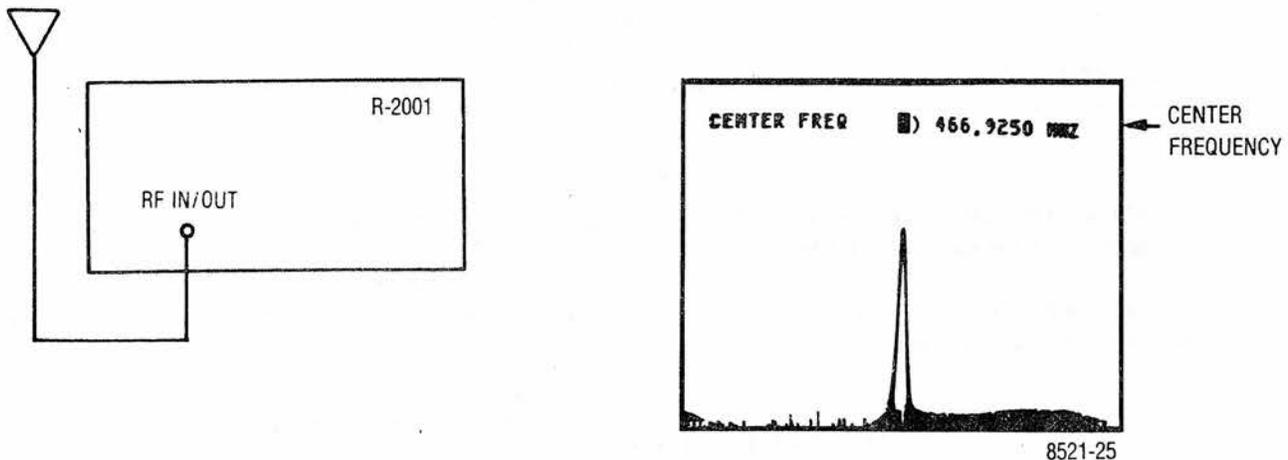
Figure 4-6. Spectrum Test Setup and CRT Display
