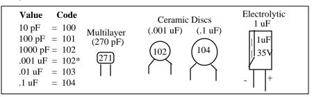
As with resistors, it's helpful to sort capacitors by type, and then to arrange them in ascending order of value. Small-value capacitors are characterized in pF (or pico-Farads), while larger values are labeled in uF (or micro-Farads). The transition from pF to uF occurs at 1000 pF (or .001 uF)\*. Today, most monolithic and disc-ceramic capacitors are marked with a three-number code. The first two digits indicate a numerical value, while the last digit indicates a multiplier (same as resistors).
