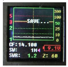
5. Pushing knob move the purple triangle to MEM, you can fast change frequency by turning the knob between MEM-0 to MEM-9. Pushing the knob for over 1 second, you can store current frequency, step, scan width into current memory bank.
