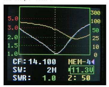
4. You can change the scan width when tune the knob and indicate purple Triangle on "SW". Push the knob for 1 second to save. FG01 will memory current CF,SW,step in next power on.
