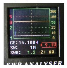
Battery indicate turns red when lower than 9.5V, must charge the battery immediately! Or will damage the battery!
