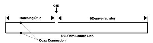
A special water-proof sealant has been applied to the coax braid and to all solder connections to prevent water migration into the cable. Heat shrink has been applied to provide more durability to the connections. The MFJ-1736 comes ready to use. However, be sure to seal all coaxial connectors against weather and moisture in normal fashion.
