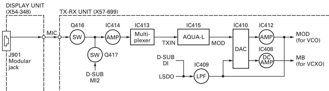
Fig. 2 Microphone and modulation level adjustment circuit
