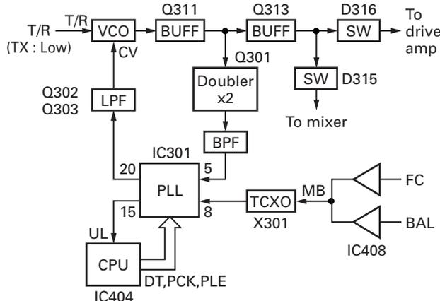
Fig. 4 PLL block diagram
