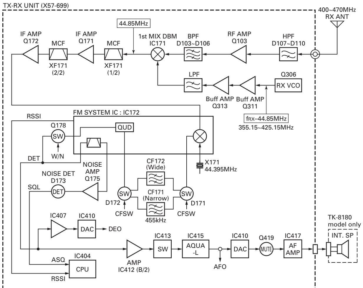
Fig. 1 Receiver circuit
