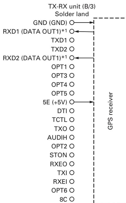
\*1 : Depending on the connected optional accessory, the DATA OUT1 may connect to either RXD1 or RXD2.
