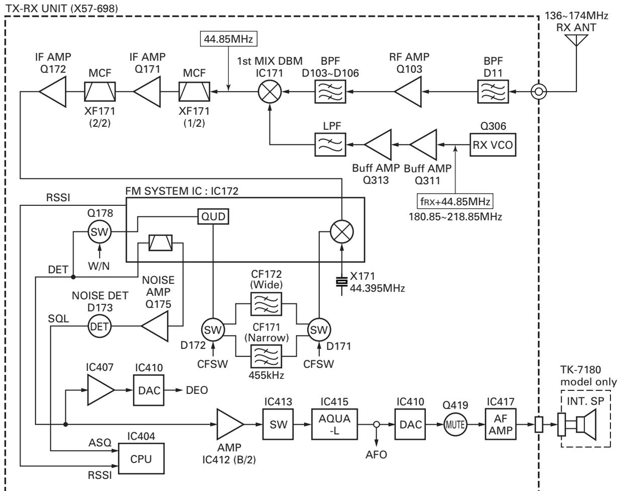
Fig. 1 Receiver circuit
