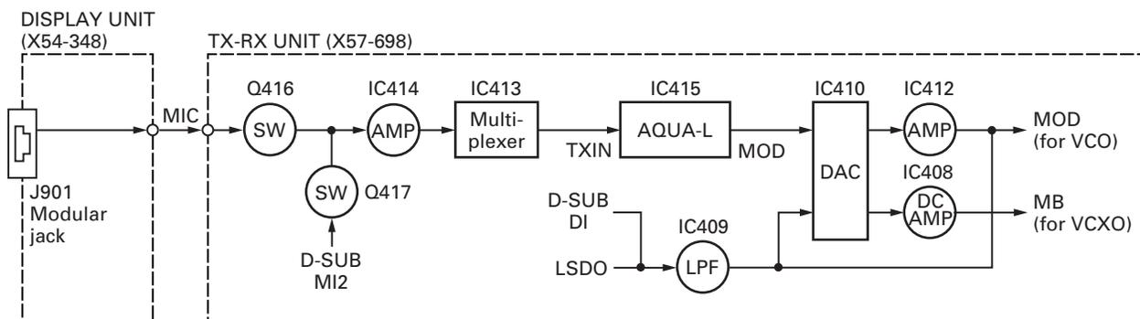
Fig. 2 Microphone and modulation level adjustment circuit
