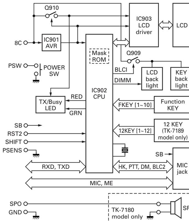
Fig. 7 Display circuit
