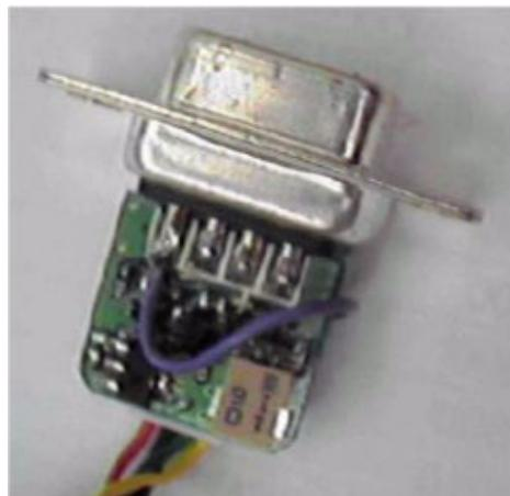
4. Install the connector cover on pin 9 of the D-sub connector.
