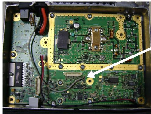
Solder the ignition line of vehicle to this pad.
