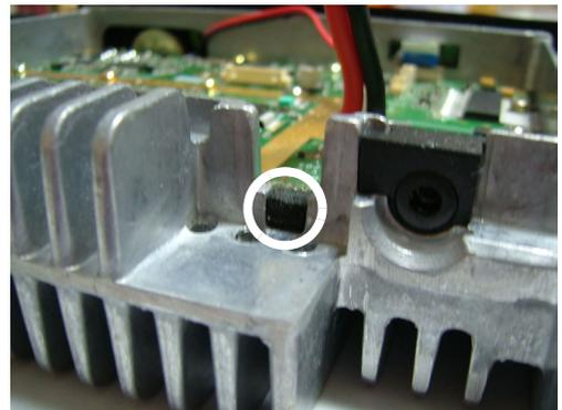
5. Dress the KCT-39 cable into the transceiver as shown in the figure.
