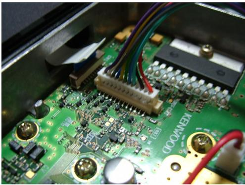
7. Connect the B connector of the KCT-39 to CN3 on the TX-RX PCB.
