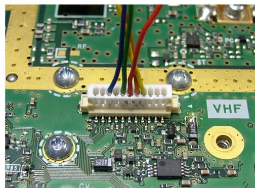
4. Connect the red wire to the hot side of the Emergency Microphone.
