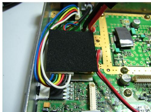
13. Put the DC cable back into place and install the shielding board, top packing, and the top case on the transceiver.
