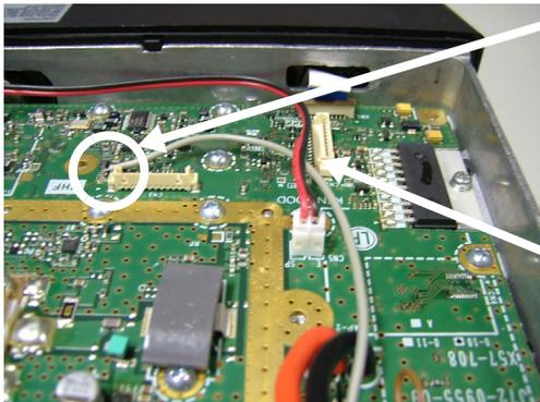
Avoid excessive stress on this soldering point.
