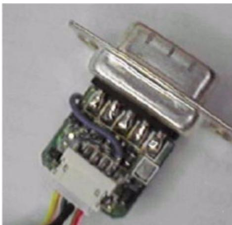
3. Connect the other end of the jumper wire in step 2 to pin 9 of the D-sub connector as shown in the figure below.
