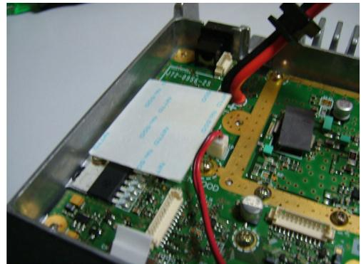
7. Peel off the coated paper of G11-4353-04 and install the KAP-2 PCB in the position shown in the figure.
