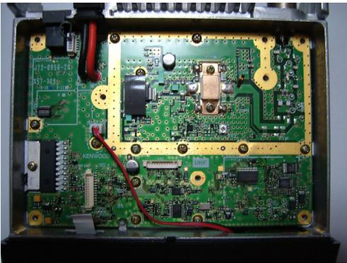
2. Connect the cable with connectors (E37-1164-05) that is used for installing the ANI Board to the CN2/ CN3 connector of the TX-RX PCB.
