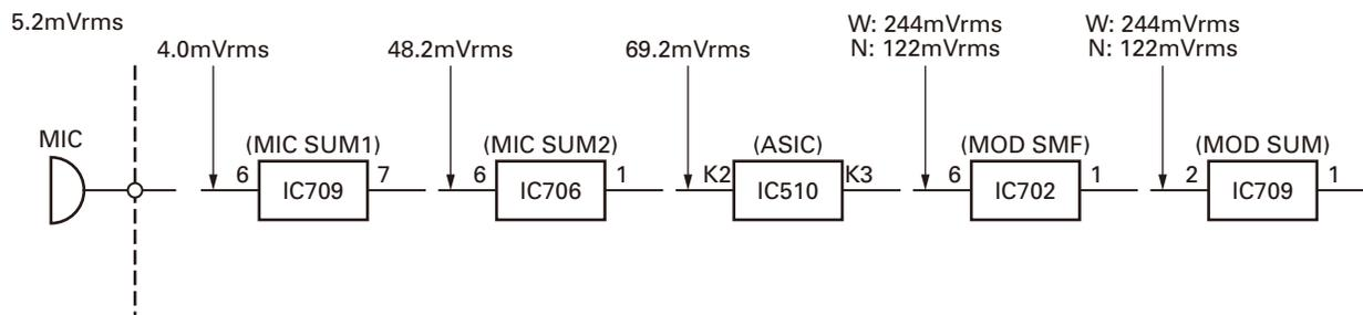
MIC input : 3kHz DEV. (Wide), 1.5kHz DEV. (Narrow) at 1kHz MOD.
