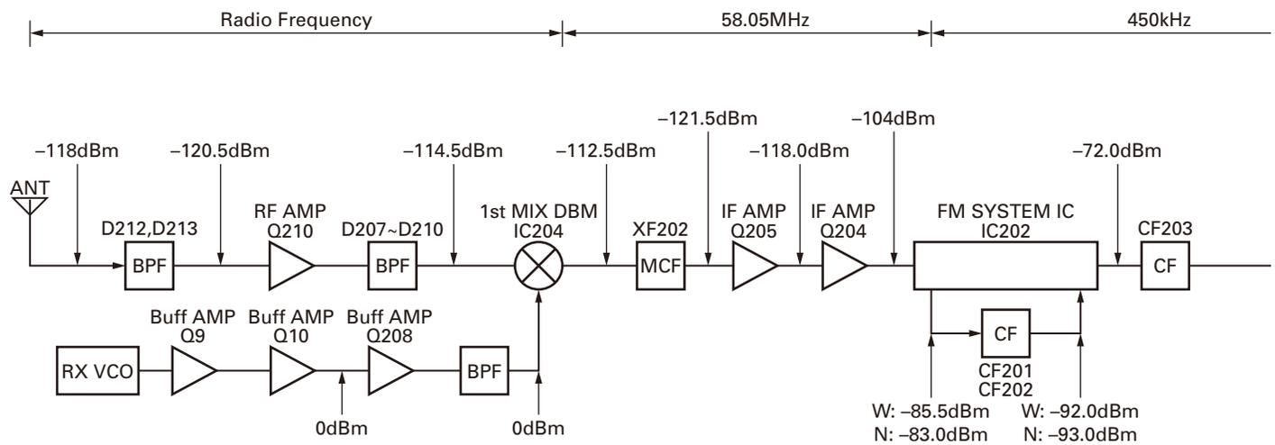
SG input level for 12dB SINAD are obtained Measured by connecting SG to each point via a 0.01 $\mu$ F capacitor.
