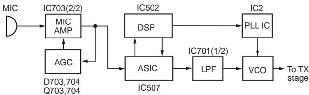
Fig. 4 Transmitter System
