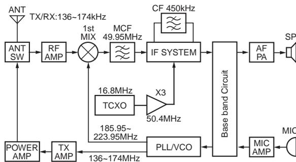
Fig.1 Frequency configuration
