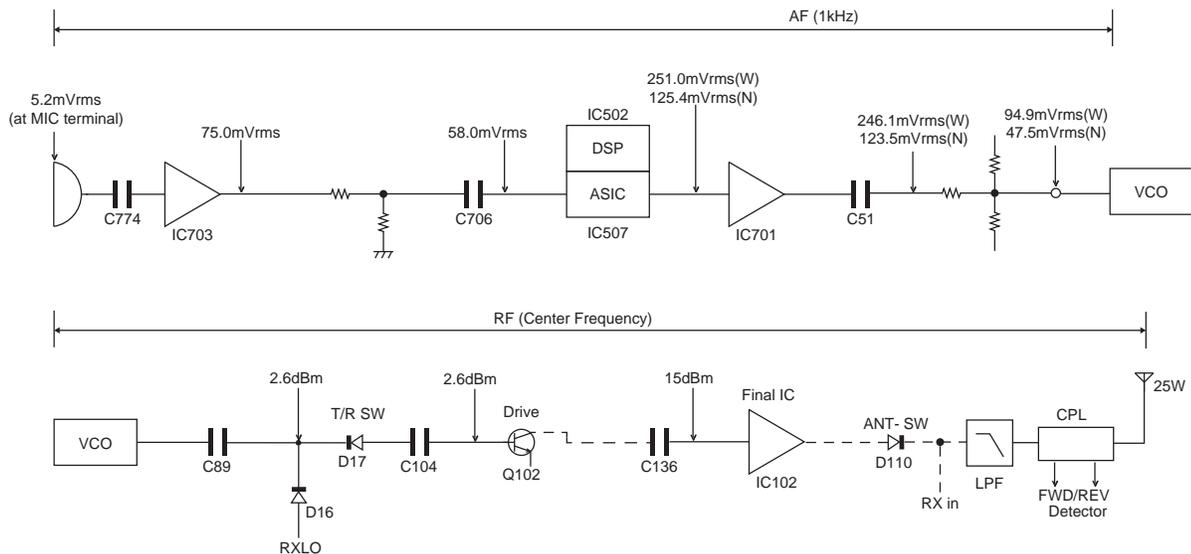
MIC input : 3kHz DEV.(Wide), 1.5kHz DEV.(Narrow) at 1kHz MOD.
