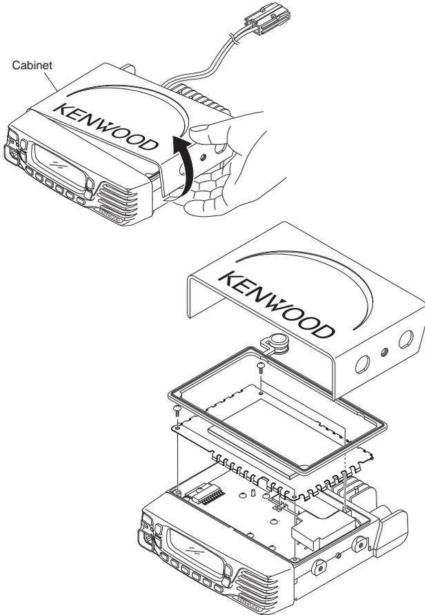
2. To remove the panel assembly, first turn the transceiver upside down. Then, insert a flat-head screwdriver into the holes of the chassis and tilt it in the direction as shown by the arrow.
