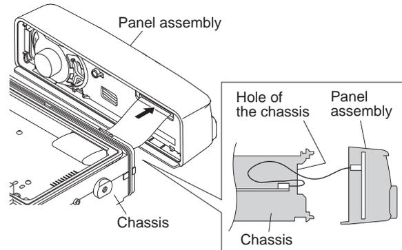
3. Fit the panel assembly into the two tabs of the chassis top side first. Then, fit the panel assembly into the two tabs of the chassis bottom side by turning the panel assembly.
