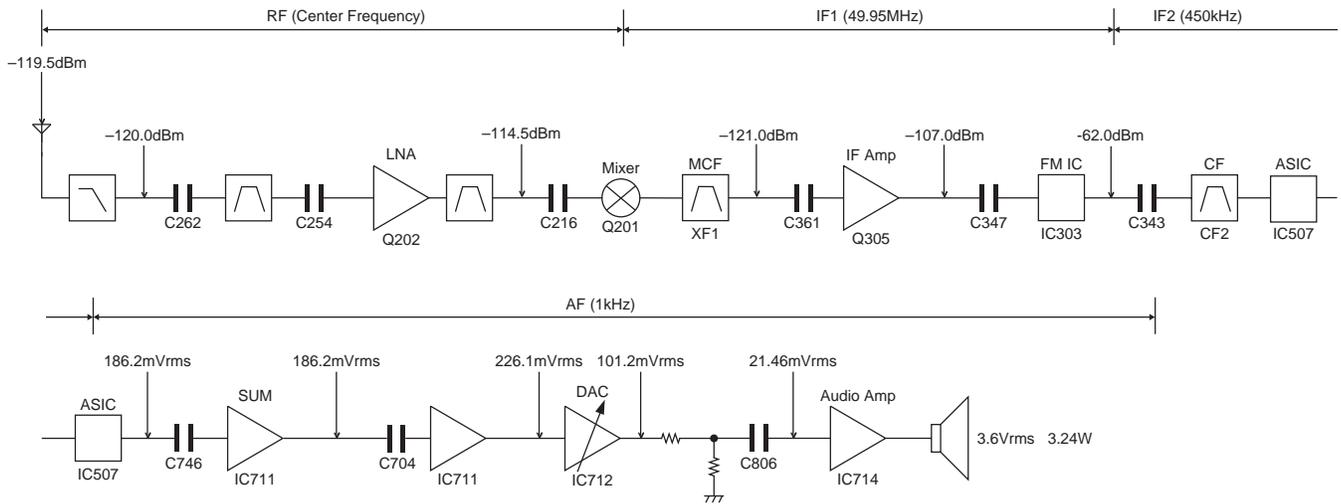
To make measurements in the AF section, connect the AC level meter. (ANT input:  $-53\text{dBm}$ , 1kHz FM, 3kHz DEV (Wide))
