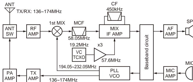
Fig. 1 Frequency configuration
