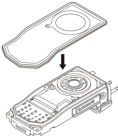
1. Place the packing on the chassis. Then, fit the chassis tightly into the groove of the packing ①.
