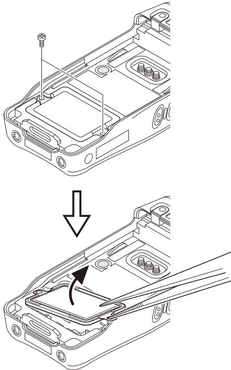
3. Remove the OPTION PCB from the connector (CN710) of the Control PCB.
