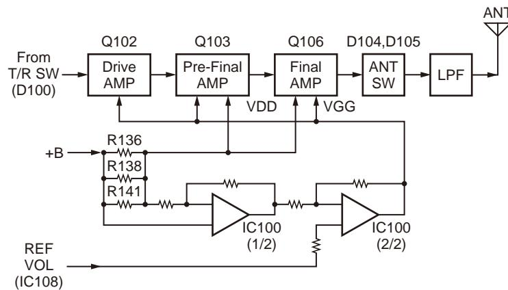
Fig. 6 Drive and final amplifier and APC circuit
