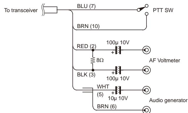
**Note:** Pin 1 (SSW) and Pin 4 (MSW) are connected to Pin 10 (GND) to active External SP and External MIC.
