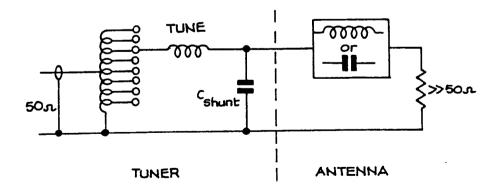
These antennas appear as a high resistance (which may be too high to be matched by the auto-transformer) in series with an inductance for lengths below  $\lambda/2$  or above  $3\lambda/4$ , and a capacitance for lengths between  $\lambda/2$  and  $3\lambda/4$ .
