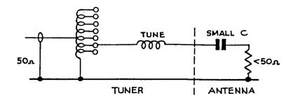
The series inductor in the tuner resonates with the series capacity of the antenna, and the RF auto-transformer matches the antenna resistance to 50 ohms.
