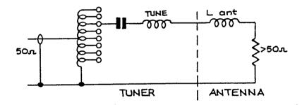
A fixed series capacitor in the tuner together with some small additional series inductance resonates with the series L of the antenna, and the RF auto-transformer matches the antenna resistance to  $50~\rm ohms$ .
