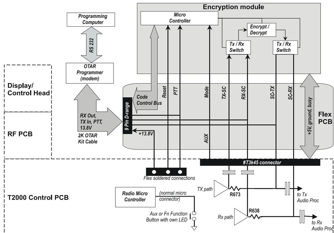
Connecting an encryption module automatically diverts the audio through the module. No link setting changes are required if a module is removed.
