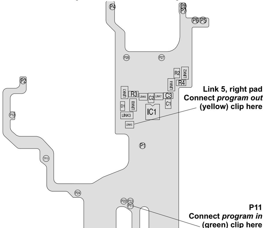
**Note:** The flex shown is 228-22592-06A. Other versions of this flex differ slightly, but the connection pads are the same. Refer to the PCB Information section.
