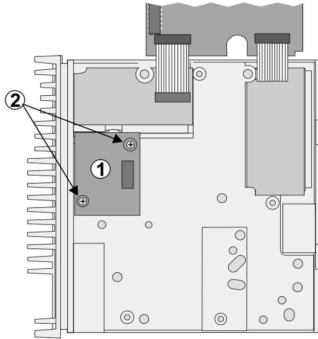
3. Fold Logic PCB back into radio chassis
