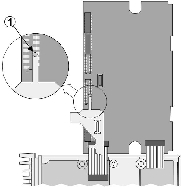
2. Gently fold flex up into position shown and plug SK1 into Logic PCB socket #T3K45
