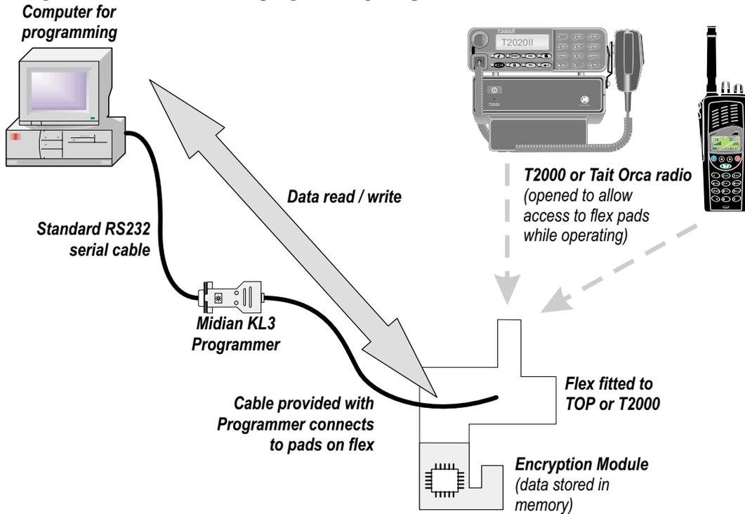
Use the cable provided with the Midian Programmer to connect the programmer to the pads on the flex circuit. See diagrams on the following pages for correct connection points.
