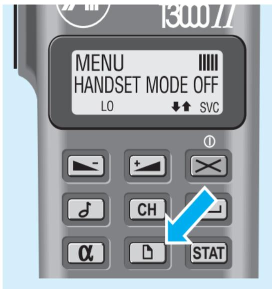
Use the cursor keys to move between menu options. Most menu options have an ON and OFF setting. To change the current setting, press the Enter (↵) key. To leave the menu options and return to normal operation press either the Menu (☰) key again or the Clear (✕) key.
