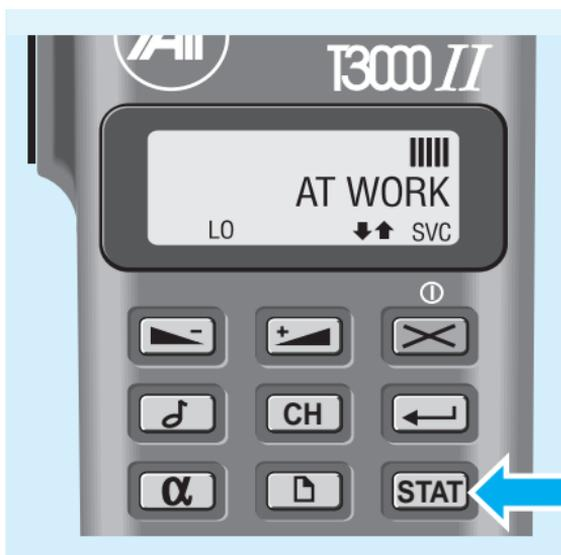
2. Press the Enter (↵) key. The label message in the display changes to its numeric value.
