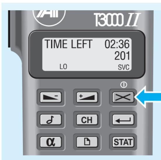
The length of a call may be limited by the network, or by your radio. Normally, your radio displays the time remaining for the call, in seconds. Depending upon the network and call type, the display may show time used, or there may be no time display at all.
