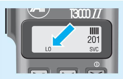
The LO indicator also appears in both Trunking and Conventional mode on calls or channels which have been preprogrammed for low power operation and cannot be cancelled.
