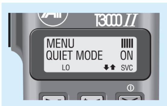
To initiate Quiet mode, use the Menu to set the QUIET MODE option ON<sup>5</sup>. (This feature can also be set by using a dialling sequence. For more information, see Appendix IV, “Common Dialling Functions”.)
