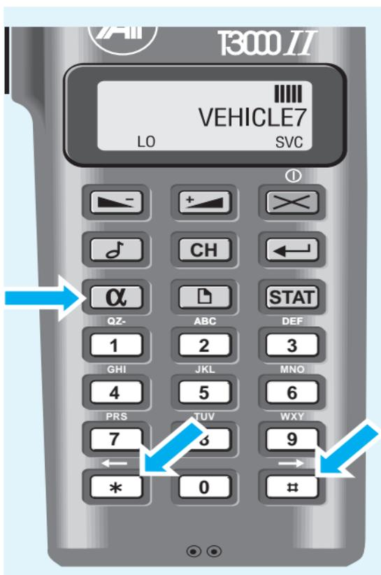
2. Locate the desired label by using the cursor keys to scroll through the list until the label is displayed or enter the label for the required party, using the keypad.
