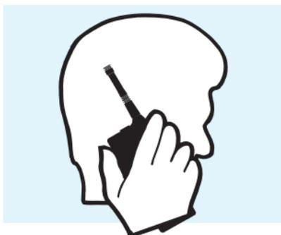
the radio operates normally. Lift it to about 15 cm from your face with the speaker beside your ear and the bottom of the radio beside your mouth as shown. Press and hold the PTT key each time you speak, as described above.
