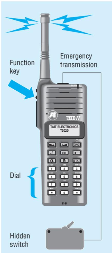
The T3020II can be set up to make an emergency call to a preprogrammed party (usually your base or dispatcher). This facility may be accessible via one of the function keys, or a switch fitted externally to the radio.
